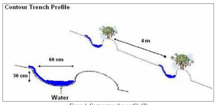
Figure 1. Contour trenches profile [2]
