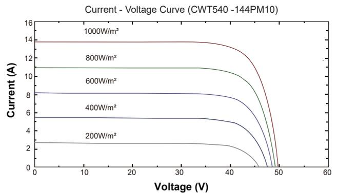
\* The specifications are obtained under the standard test conditions: 1000W/m<sup>2</sup> solar irradiance, 1.5 Air Mass and cell temperature of 25°C. Measurement uncertainty for all panels is 3%. The actual transactions will be subject to the contracts. These parameters are for reference only and it is not a part of the contracts. The technical specifications in this document may vary. For more information, refer to the "Installation Manual".
